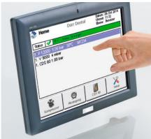
Visual display for monitoring all functions from a central control station, e.g. in the technical room
