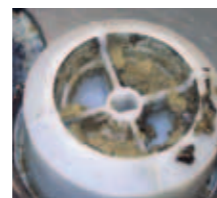
Centrifuge drum, performance hindered by sludge
